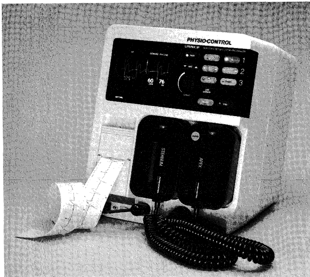
Figure 1-1 LIFEPAK 9P defibrillator/monitor/pacemaker
